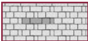
Pattern 5 – Per 100 sq. ft.: 150 Standard Tapered, 75 Half, 75 Jumbo
