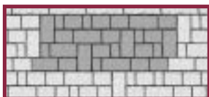
Pattern 7 – Per 100 sq. ft.: 124 Standard Tapered, 73 Half, 94 Jumbo
