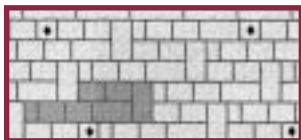
Pattern 3 – Per 100 sq. ft.: 160 Standard Tapered, 42 Half, 80 Jumbo
