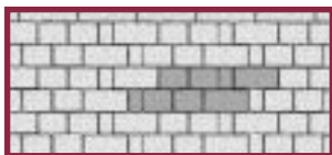
Pattern 6 – Per 100 sq. ft.: 150 Standard Tapered, 75 Half, 75 Jumbo
