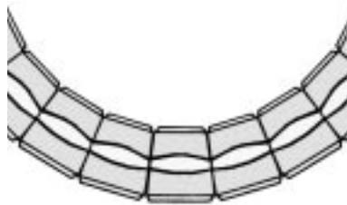
The minimum radius for a curve using Stack Stone is 21" inside and 29" outside. For inside curves either the larger or smaller face can be used for the face of the wall. For outside curves, only the larger face can be used for the face of the wall.
