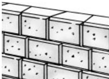
Coping units, which form the finishing course, must be secured to the top of the wall with an adhesive. A Coping unit may replace a Standard unit anywhere within the wall as long as it is not placed above or beside any other Coping unit.
