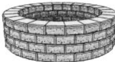
Walls constructed without soil within 8" of the top are considered to be free standing. For free standing walls it is necessary to place adhesive under the top two courses. When constructing circular walls the minimum number of pieces per ring is 23.
